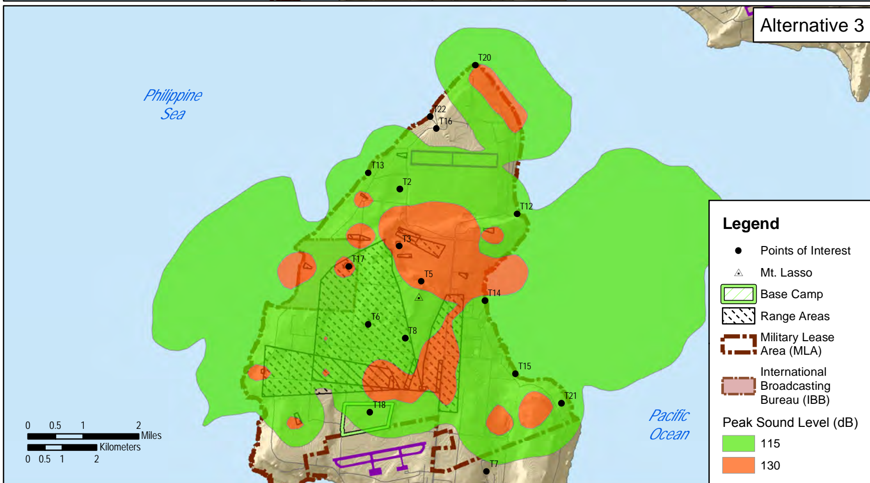
Figure 4.5-4. All Tinian Alternatives Large-Caliber Peak Noise Levels under Neutral Weather Conditions (Peak)
